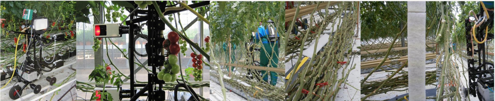
The Crop Adapted Spraying (CAS) sprayer sprays only there where it is necessary. The CAS-sprayer uses a sensor to detect the tomato stem and will spray it when a disease is to be controlled.
